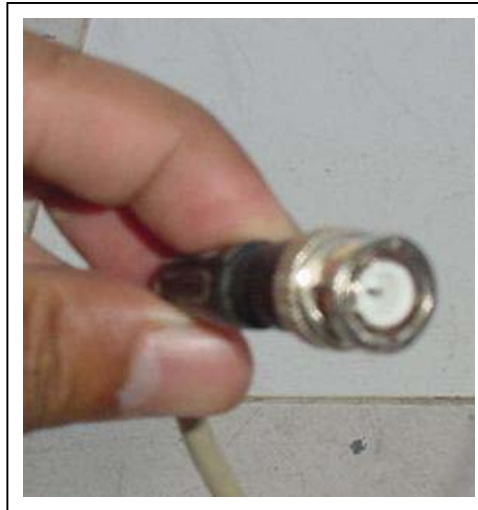
Gambar 2. Connector BNC terpasang di Cable RG-58
